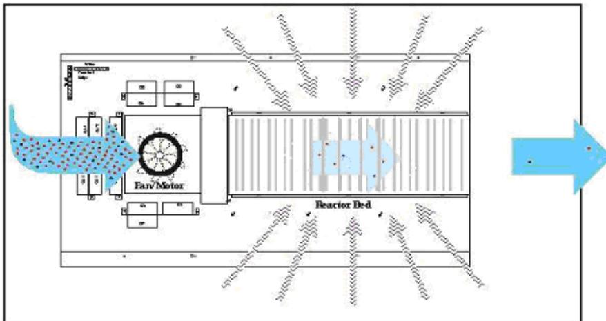
Contaminated air is drawn into the AiroCide system by the fan. It passes over the reactor bed where it is immobilized on the TiO<sub>2</sub> catalyst and treated with UV-light until it is completely broken down to gaseous products. The combination of TiO<sub>2</sub> catalyst and UV-light has been shown to destroy hydrocarbon bonds in allergens, airborne organisms and VOC's.
