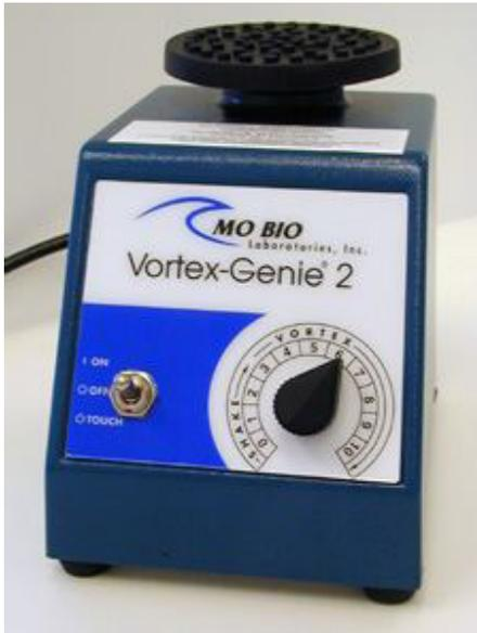
The Vortex Genie® 2 Vortex blends fluids quickly and thoroughly with a true vortex action that prevents spilling, even when tubes are uncapped. It is capable of ranges from gentle yet thorough shaking action to extreme vigorous vortexing depending on the attachment chosen.
