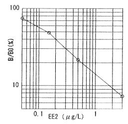
Samples containing EE2 within the dynamic range between 0.05 $\mu$ g/ L and 3 $\mu$ /L. can be directly applied to assay after filtration.
